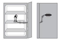
Place the buffered probe in the center of the chamber near vaccine but away from vents, coils, cooling plates, walls, ceilings, and floors. We recommend securing the probe in place. Requirement
