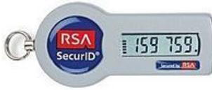
Your MIDIS Key Fob has a 6 digit number that changes every 60 seconds. This number is the Key Fob tokencode. The tick marks to the left of the number represent how much time is left before the number will change. There is one tick mark for every 10 seconds left. When all the tick marks are gone, then the number will change. For best results, enter the Key Fob tokencode and click on the Logon button before all the tick marks are gone.
